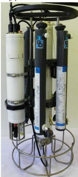
The NISKIN bottles are closed in sequence starting from bottle 1 to bottle 5. The MISS integrates a rechargeable battery pack to power the sampling system and optionally the interfaced CTD.
