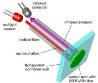
to the excellent luminescence brightness of the REDFLASH indicator, the actual sensor matrix can be now prepared much thinner, leading to fast response times of the oxygen sensors.
