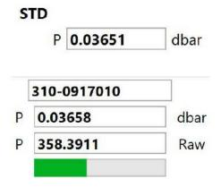
• **Pressure Calibration Points Section,** that shows the number of acquired pressure calibration points, the button to execute a new acquisition of calibration point and the button to start the realtime pressure data acquisition. The acquired calibration point will be saved to a file txt in the session's folder.
