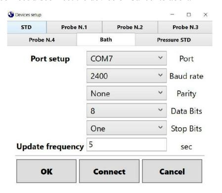
• **Pressure STD Section**, that allows the user to connect/disconnect the Pressure STD (*Paroscientific Digiquartz Laboratory Standard 745*) to the program. Select the port, the baud rate, the parity bit, the data bits, the stop bits and the update frequency. Click the button Connect/Disconnect to connect/disconnect the device or Cancel to abort.
