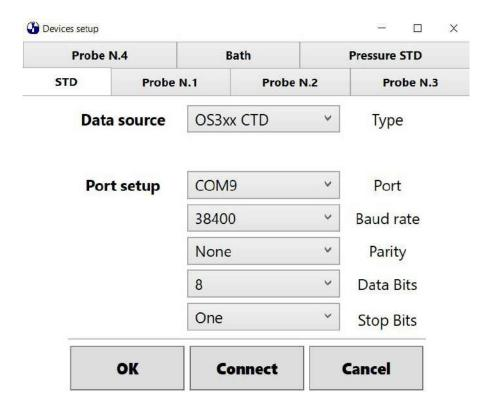
• **Probe Section**, that allows the user to connect/disconnect the probe to the program. Select the source type, the port, the baud rate, the parity bit, the data bits and the stop bits. Up to four probes can be connected to the program at the same time. Click the button Connect/Disconnect to connect/disconnect the device or Cancel to abort.
