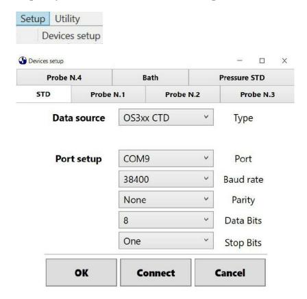
3. Go to **Probe N.1** tab and set the source type, the port, the baud rate, the parity bit, the data bits and the stop bits. Then click the button **Connect** to connect the device. Repeat the operation if you need to connect more probes. Up to four probes can be connected to the program at the same time.
