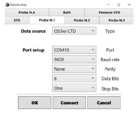
• **Bath Section**, that allows the user to connect/disconnect the bath (*Hart Scientific High Precision Titanium Bath 7012*) to the program. Select the port, the baud rate, the parity bit, the data bits, the stop bits and the update frequency. Click the button Connect/Disconnect to connect/disconnect the device or Cancel to abort.
