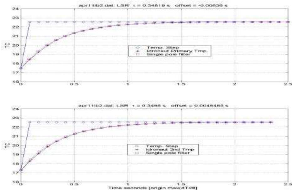
Figure 5 a-b: Plot of response of Idronaut primary temperature probe (\*) (upper panel) and Idronaut 2nd temperature probe (\*) (lower) both panels show step temperature change ( $\diamond$ ) and model response ( ) for time constant ( $t$ ) shown.
