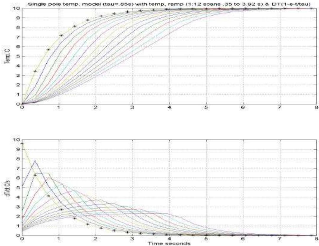
Figure 6 a-b Upper panel is sensed temperature versus time for longer ramping intervals and lower panel shows maximum temperature gradient delayed increasing time intervals until temperature ramp end
