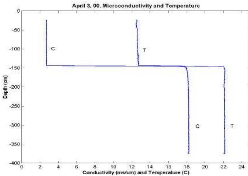
Figure 2a Profiles obtained with the microstructure sensors of conductivity and temperature through the double-diffusive plunge tank from April 3, 2000.
