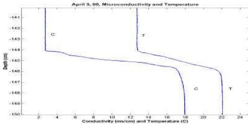
Figure 2b. Expanded view of the interface between the two layers for the April 3 run. The interface is little more than 1 cm thick; the temperature gradient is approximately  $700^{\circ}\text{C}/\text{m}$ .
