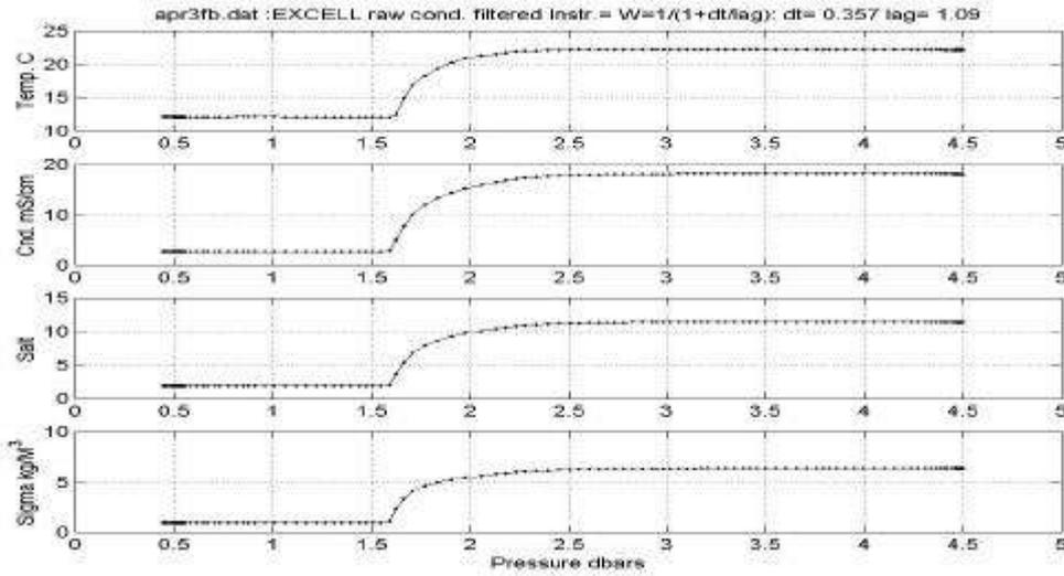
Figure 7 a-d Four panel plot of temperature, conductivity, salinity, and density versus pressure from the 2<sup>nd</sup> April 3, 2000 plunge of EXCELL # 1321. The instrument default filtering with  $t=0.93$  s has been applied to conductivity and pressure.
