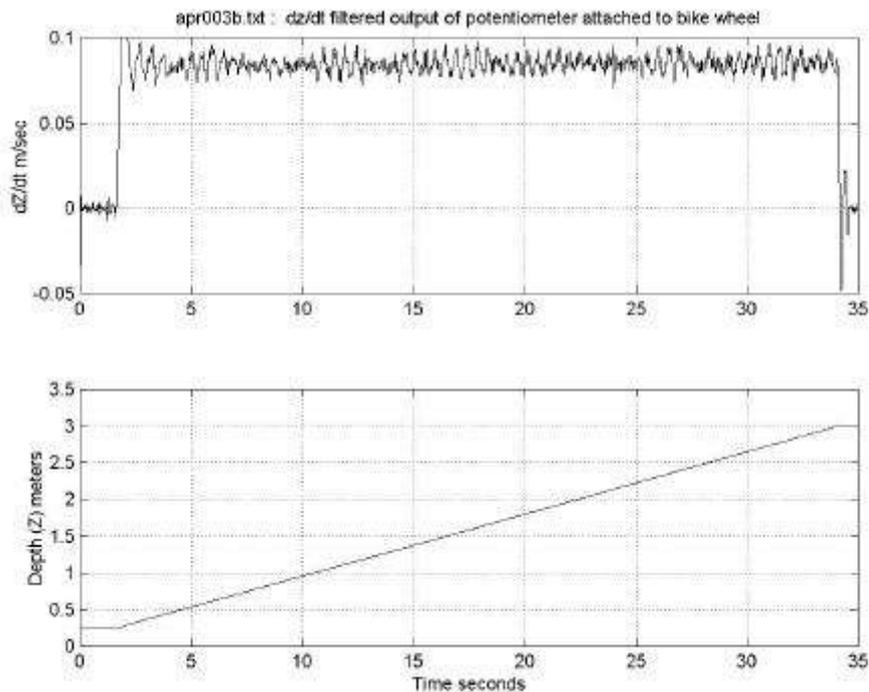
Figure 2 c & d Displacement (lower) and filtered drop rate (upper, oscillations are filter artifact) versus time for a run on April 3, 2000.
