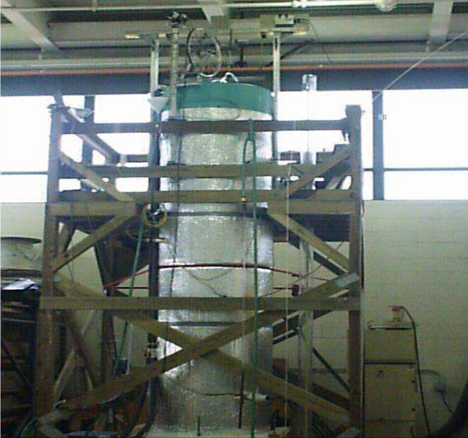
Figure 1. The double-diffusive interface tank in the Clark Annex high bay. The PVC tank stands 4.7 m high and has an internal diameter of 91 cm. Aluminumized bubble wrap provides insulation. A stairway at the rear provides access to the working platform. The speed of the bicycle wheel controls the fall rate of sensors through the sharp interface. The counter weights travel within the clear tubing to the right.
