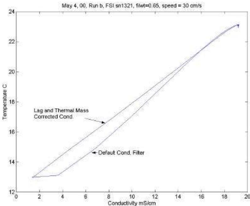
Figure 9.b A higher speed run ( $\sim 30$  cm/s) shows the need for lagging of the conductivity record relative to temperature, which corrects the C-T curve at the beginning of the interface (low C, T values). The thermal mass correction (with  $a=0.4$ ,  $b=0.6$ ) serves to straighten the C-T curve at high C, T values, where the sensor has entered the lower warm, salty layer.
