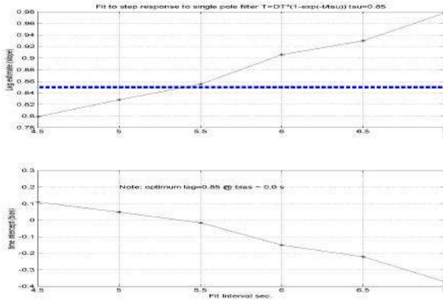
Figure 4 a-b Illustration of bias =0.0 time offset producing optimum response time estimate for exponential data simulation using  $\tau=0.85$  s, fit for slope =  $1/\tau$  (upper) and bias= time offset (lower panel) plotted versus fitting interval in seconds (for 2.8 hz sampling interval).
