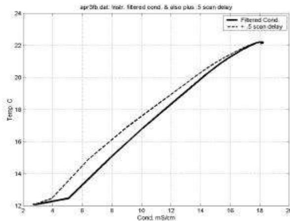
Figure 8a, gives a lag  $t = 1.09$  s (model response is squares) while temperature observations are indicated by asterisks (\*). Figure 8b “Figure of merit” plot of C versus T. (Solid) is observed instrument conductivity while (dashed) has a 0.5 scan (0.179 s) delay added to the conductivity, since its external field senses the interface prior to the thermometer.
