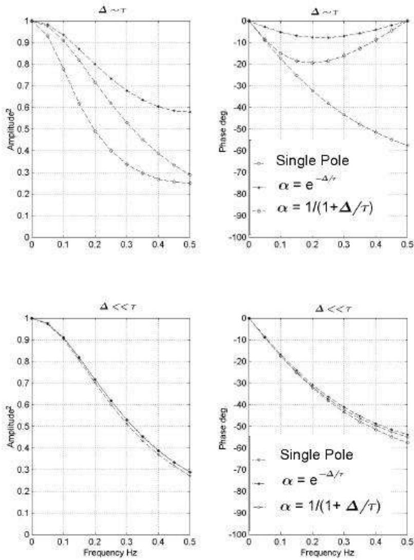
Figure A1 a & b: (upper 2 panels) Evaluation of equation 12 for the amplitude squared and equation 14 for the phase. This represents the case where the sample interval ( $\Delta$ ) and lag ( $\tau$ ) are approximately equal. Figure 10c & d (lower 2 panels) Evaluation of equation 4 for the square of amplitude response and equation 3 for the phase. This represents the case where the instrument sample interval ( $\Delta$ ) is much smaller than the lag ( $\tau$ ).
