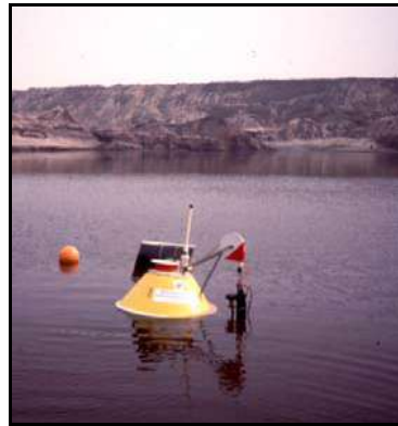
Figure 1 Automatic profiling probe (Idronaut Srl – Brughiero (MI) Italy); data acquisition and data transfer controlled by radio modem; parallel measurements of fluorescence, turbidity, pH, ORP, DO and el. conductivity against depth
